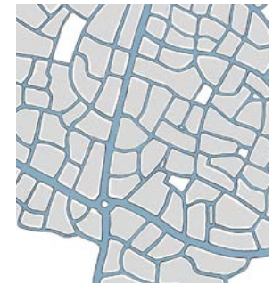
Figure 135: The differences between a disconnected and connected network of streets as illustrated in the National Model Design Code. Connected streets help to reduce walking distances and set a long-lasting framework for movement.
