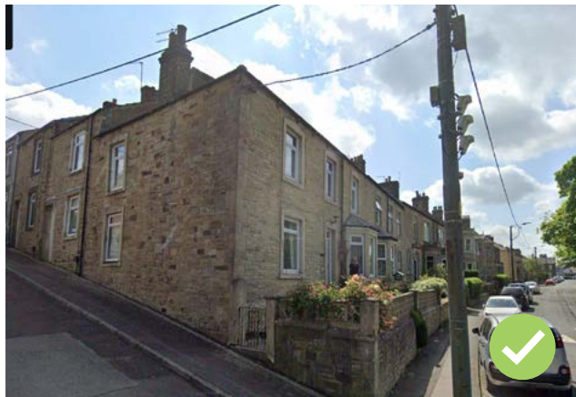
Figure 20: Terraces that positively respond to topography with stepped or sloped rooflines. Along main routes, small setbacks with strong boundary treatments allow space for front gardens, and positive visual continuation of frontages.
