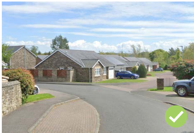
Figure 36: A change in road surface helps to demarcate the road hierarchy and parking areas. The access lane and on-street parking bays are paved to indicate a different character/use.
